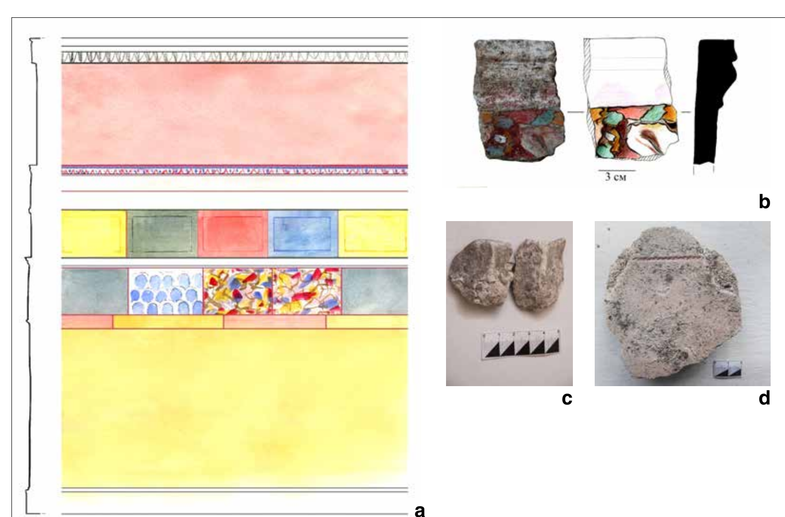
4. (a, b) Images of cross-section from a red colored fragment, (c) images of the fragment and (d) a fragment with a red paint layer and at least three plaster layers with different morphological characteristics (marked I, II, III).
